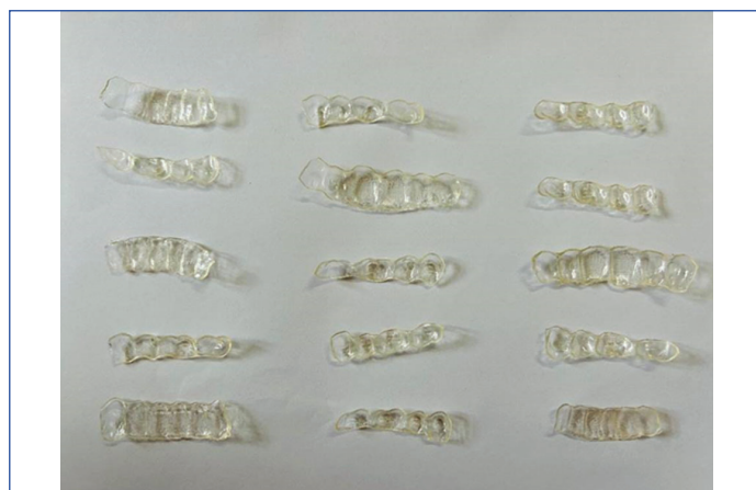
[Table/Fig-8]: Aligners after immersion in carbonated drinks for 2 weeks.
