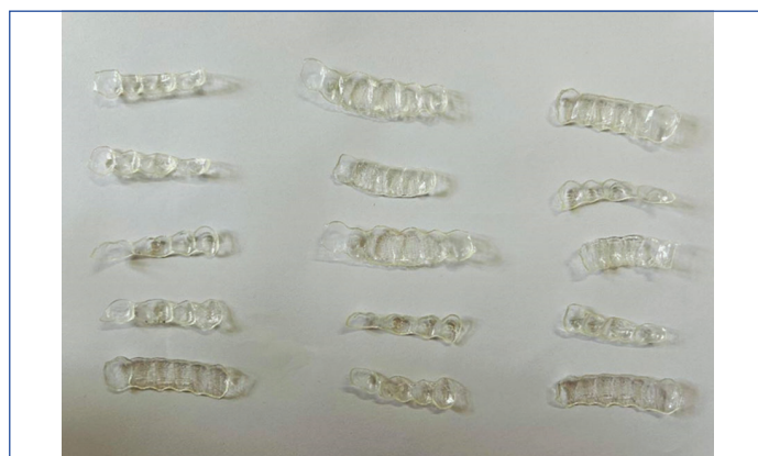
[Table/Fig-10]: Aligners after immersion in distilled water for 2 weeks.
